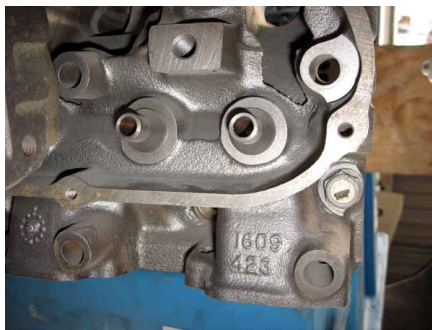
425 Head Casting Number On Exhaust Port
