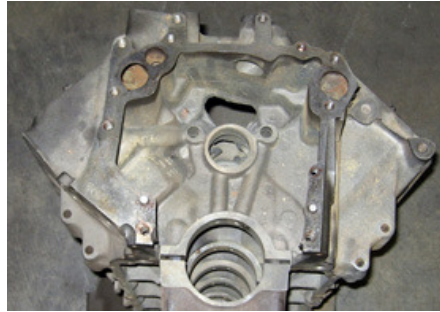
425 Block Front View and 425/ 368 Timing Cover
