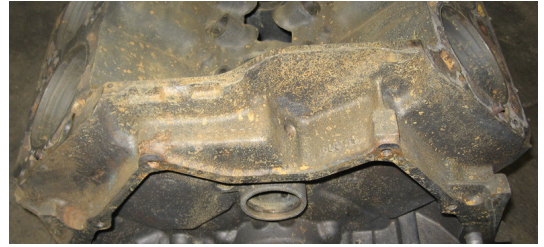
425/368 Block Rear Top View => Note Box shape on Driver's side, not present on 472/500 block.
