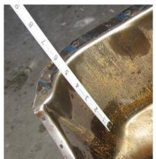
Bend the tube - Install the dipstick, set your square on the oil pan rail, and set up your tools for rotating the crank. You want to make sure that when you are done bending the tube, you meet 2 conditions - 1, the rotating parts do no hit the dipstick or tube, and 2 - the full mark is roughly 5" up from the oil pan gasket surface on the block.
